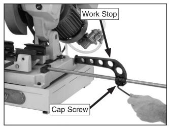
Figure 12. Work stop adjustment.
